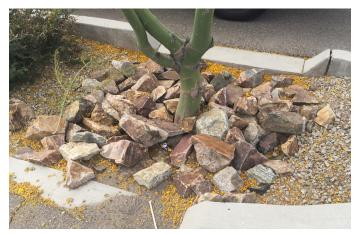
Fig. 15. Parallell curb cuts in a small planting island and riprap on top of the tree root zone.
