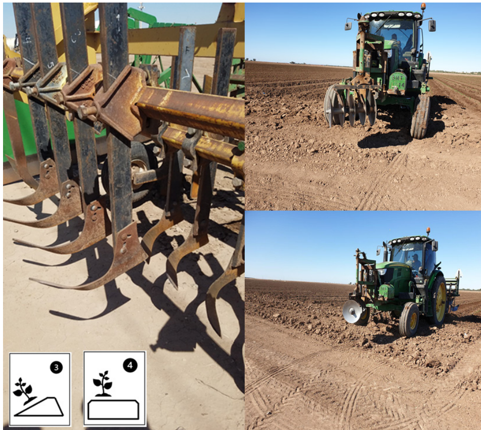
Figure 21. Continuous seeding and tillage of asymmetric beds either requires two sets of differently orientated implements that are raised or lowered to match field orientation ('banana sweeps' on image left), or equipment that is rotated 180 degrees to match field orientation (pitched disks on image right) (Coronation Peak, 2020 & SMT Melon Company, 2020).
