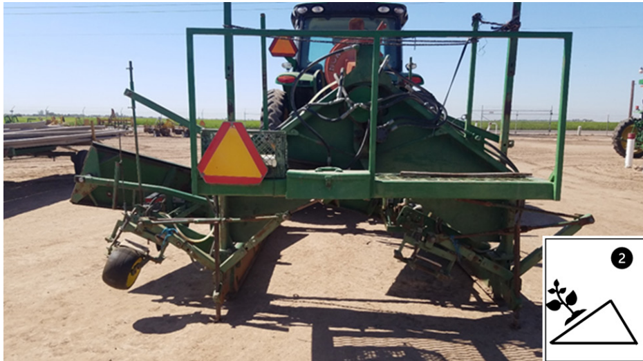
Figure 5. Rear view of a Yuma bed planter used to shape and plant angled raised beds (Coronation Peak, 2020).
