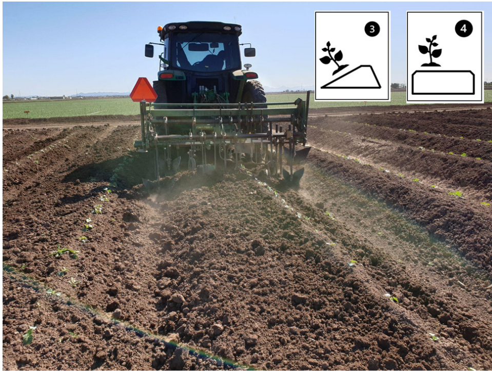
Figure 11. Offset cultivation during the 'capping' pass (SMT Melon Company, 2020).
