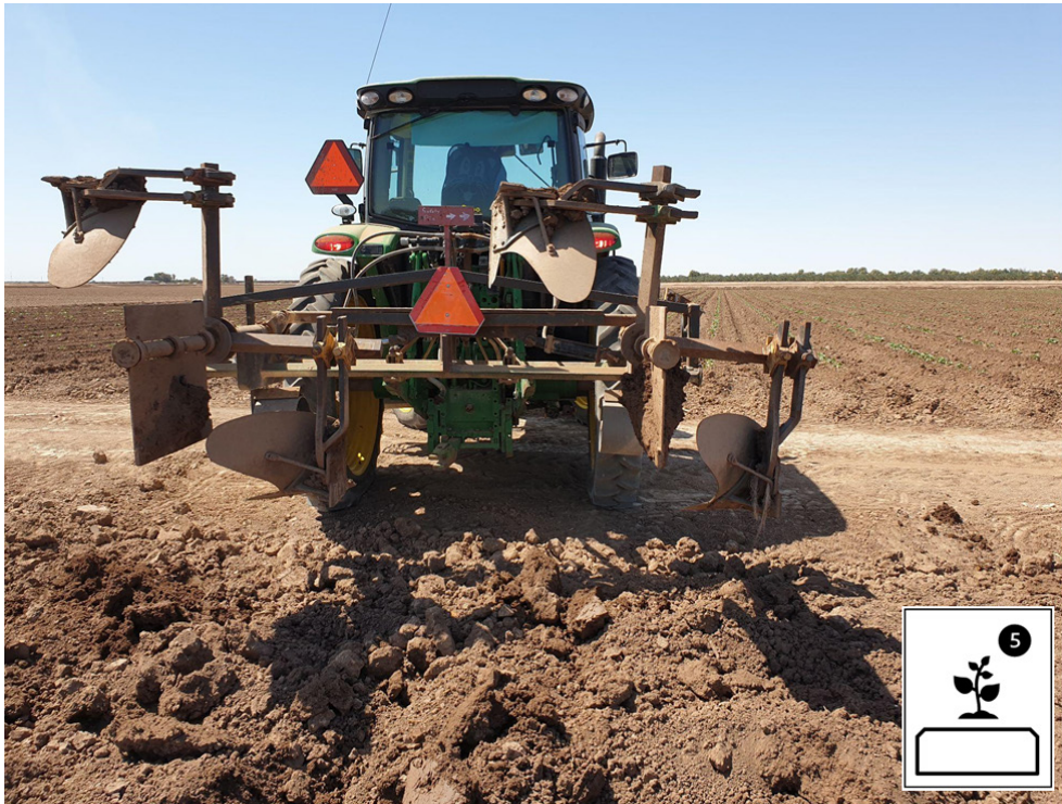
Figure 15. Ground is worked to center the seed line in the middle of the bed. Two sets of implements are set up at different orientations, which are alternatively rotated to account for asymmetrical field layout (SMT Melon Company, 2020).
