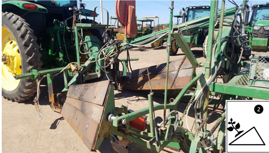
Figure 7. Left-side view of a Yuma bed planter used to shape and plant angled raised beds. The planter has two blades and vacuum planter units, so that two beds may be seeded at the same time. Equipment is rotated after each pass to account for field asymmetry (Coronation Peak, 2020).
