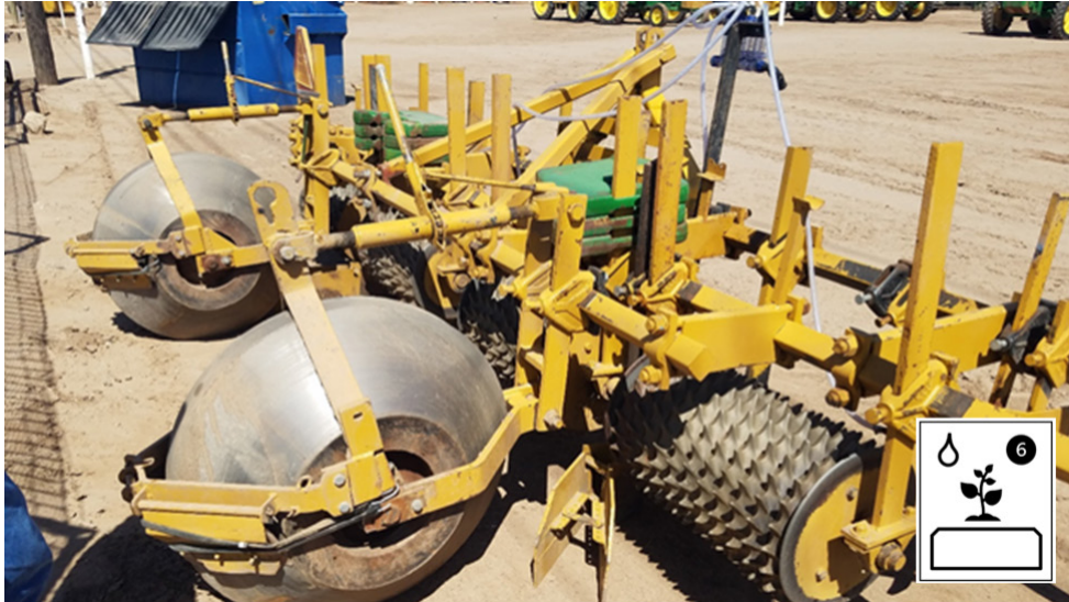
Figure 17. Cultipacker with ring rollers, "wobble tails", and bolas used to smooth newly formed bed tops and compact the furrow (Coronation Peak, 2020).
