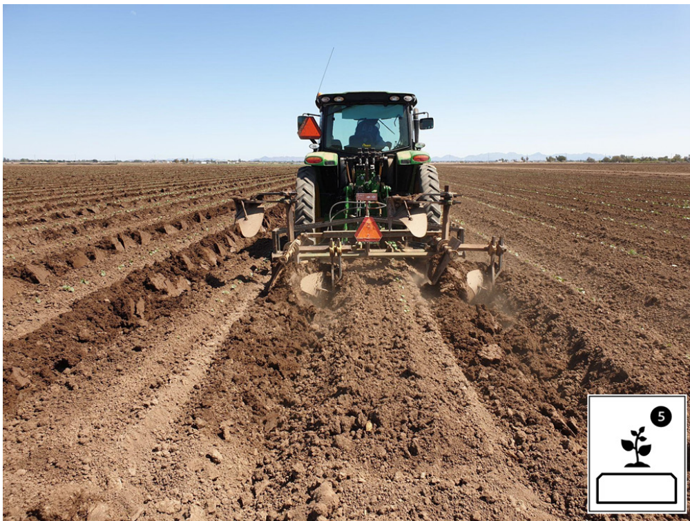
Figure 16. Beds are remade around a newly centered plant line with rotating moldboard plows (SMT Melon Company, 2020).
