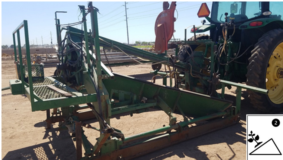
Figure 6. Right-side view of a Yuma bed planter used to shape and plant angled raised beds (Coronation Peak, 2020).
