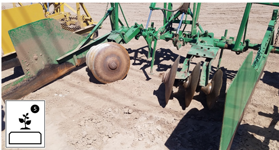
Figure 14. Pitched disks used to push soil to the edge of the plant-line on the north side of bed and rebuild the furrow around the newly centered plant-line (Coronation Peak, 2020).
