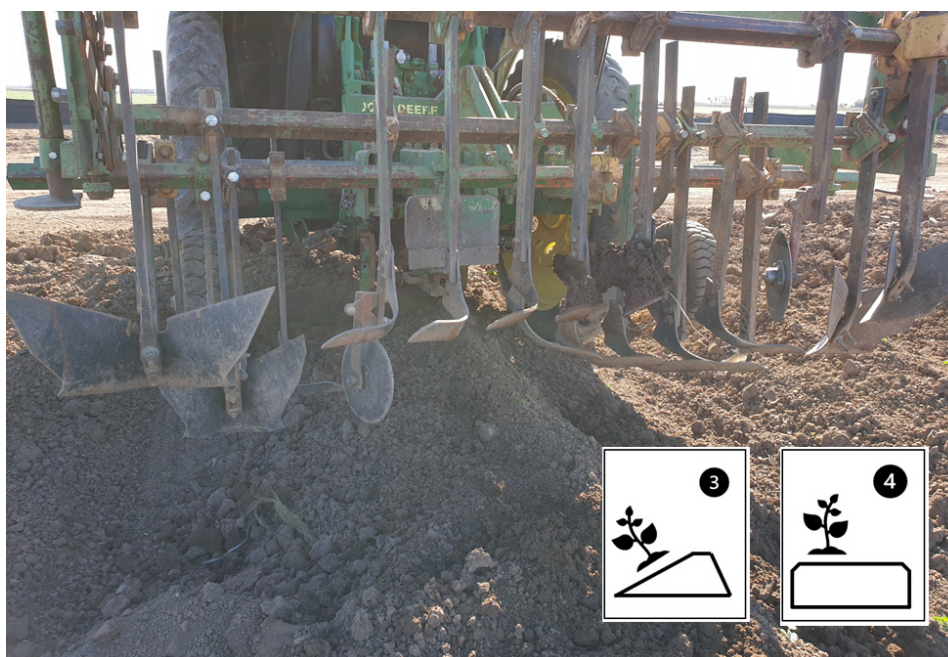
Figure 10. Banana sweeps and disks used to evenly distribute the soil on the north side of the plant-line during the 'capping' pass. Two sets of implements with different orientations are alternatively raised or lowered to account for asymmetrical field layout (SMT Melon Company, 2020).
