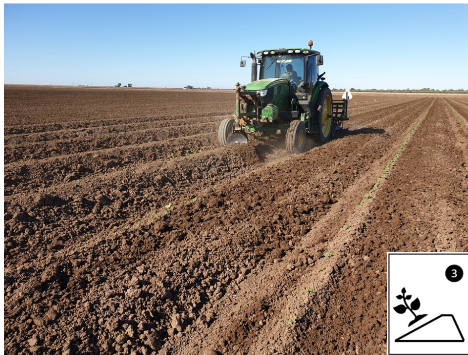
Figure 9. Bed tops are 'capped' by pushing soil to the north side of the bed with a set of adjustable pitched disks that rotate to accommodate field asymmetry (SMT Melon Company, 2020).
