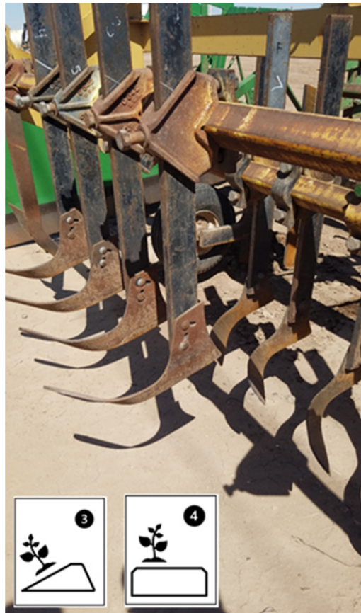
Figure 13. During the 'shaping' stage the soil on the north side of bed is further broken up and moved to the north side of bed with two sets of 'banana sweeps' that are alternatively raised and lowered to fit asymmetric field conditions.
