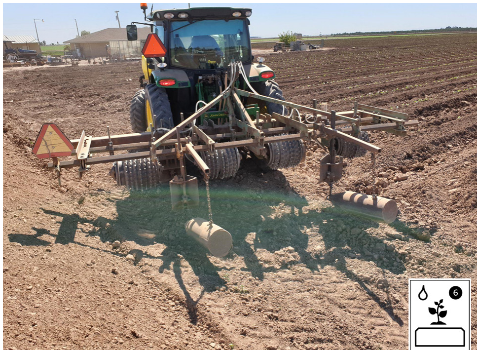
Figure 18. Cultipacker with ring rollers, shanks, and weights are used to clean the soil around the plant line and compact the furrows (SMT Melon Company, 2020).
