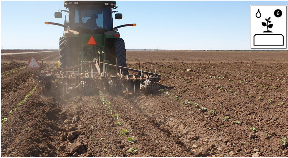
Figure 19. Cultivator used to smooth bed tops and compact furrows (SMT Melon Company, 2020).
