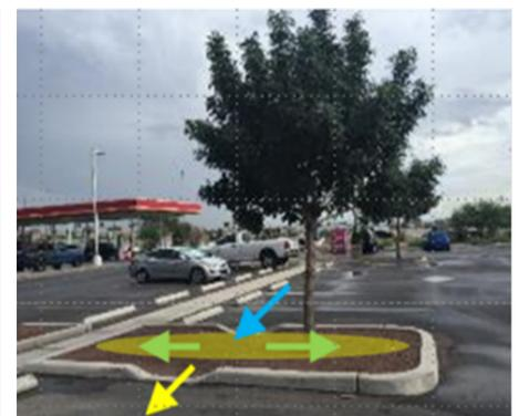
Fig. 25. Water harvesting in this planter is not effective and can be optimized by lowering the soil surface level.
