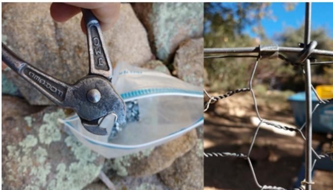
Figure 7: J-clip pliers with uninstalled j-clip (left) and installed j-clip tying poultry wire to woven wire fence (right) (Picture by Jeff Schalaus)
