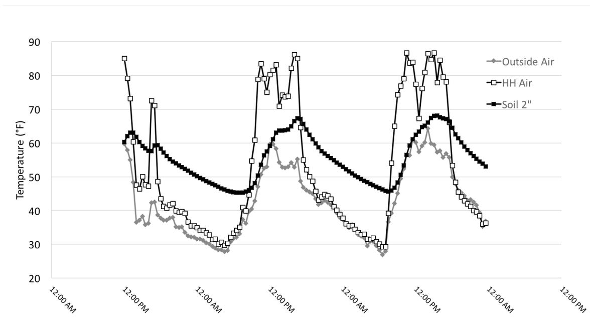
Fig. 6. Outside air temperature and soil and air temperature in a hoop house (HH) during a freezing event in Tucson, Arizona.
