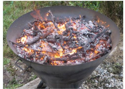
Figure 8. Japanese kiln (left). Source: [www.ithaka-journal.net/86](http://www.ithaka-journal.net/86). Biochar is produced in the pyrolysis zone where less air is available (center). Source: Image by L. Wardell. Cone with coals -- wood layer is added when the top layer begins to coat with ash (right). Source: [www.ithaka-journal.net/86](http://www.ithaka-journal.net/86)
