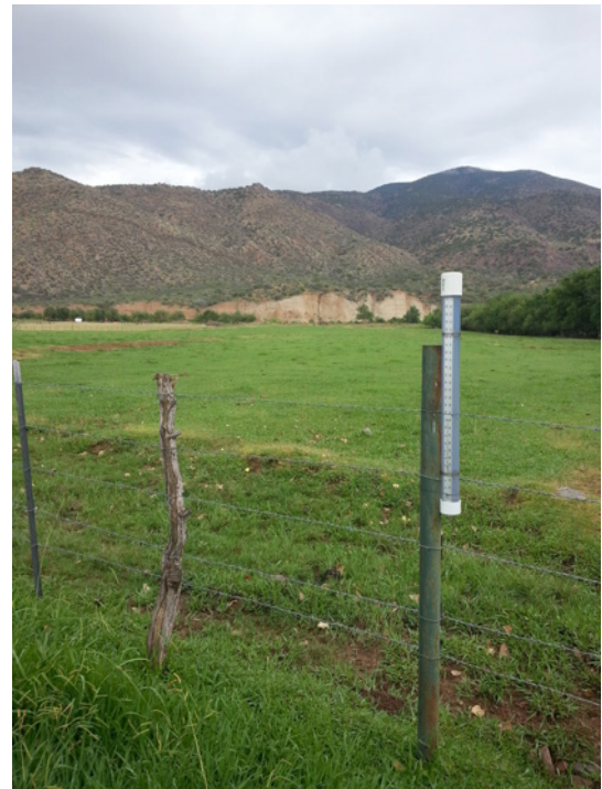
Figure 1. Clear PVC rain gauge (photo courtesy of J. Lyman)
