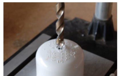
Step 2a – Drill out drain hole
