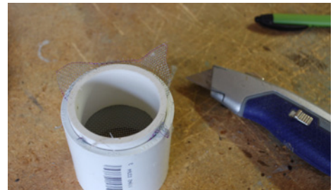
Step 5f – Trim excess using utility knife
