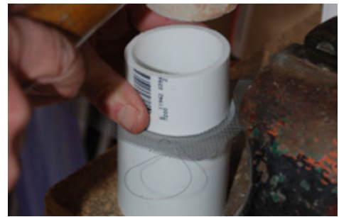
Step 5e – Tap PVC section into coupler
