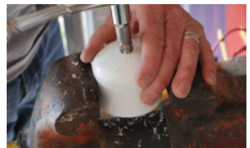
Step 2a – Create threads with tag
