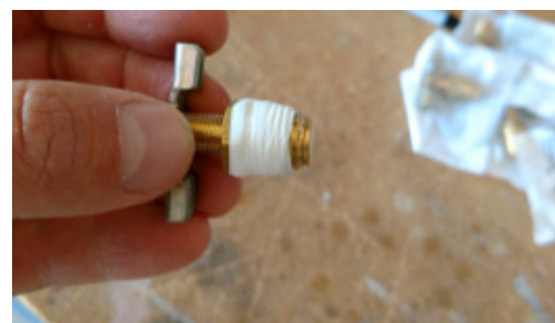
Step 4a – Wrap valve with thread sealing tape
