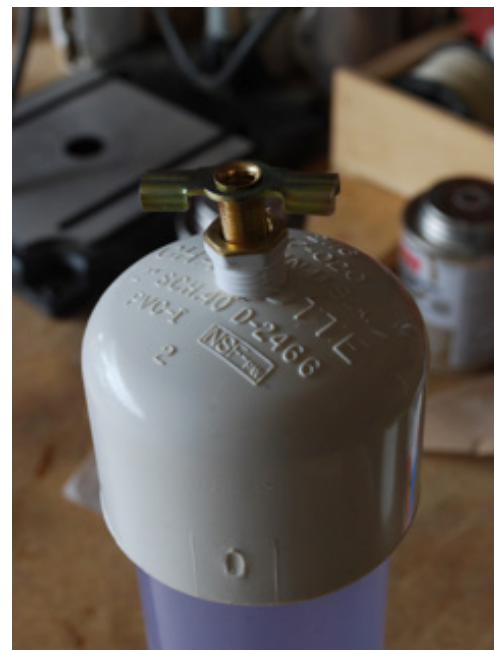
Step 4a – Wrap valve with thread sealing tape
