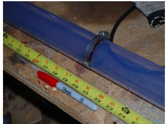
Step 1a – Mark and cut pipe to length
