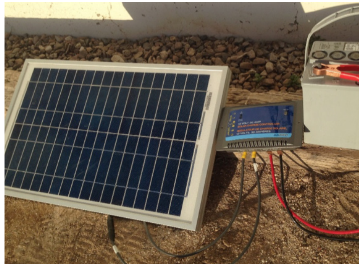
Figure 4. A solar module connected to a charge controller and battery. The controller monitors the “state of charge” (SOC) of the battery, preventing overcharging from the solar module.
