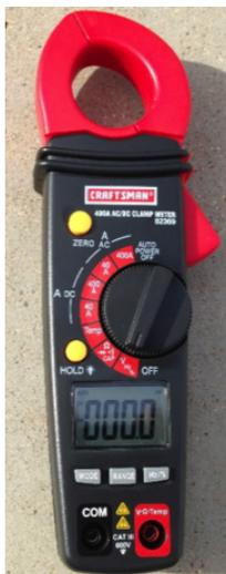
Figure 3. Example of an AC/DC Clamp-On Meter. This model shows no leads connected to the meter. This style meter may be used to measure voltage and amperage. Source: Author
