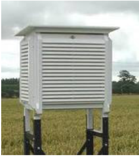
Figure 13. The Stevenson Screen (left) and the 12-plate Gill shield (right) are used to protect temperature sensors from radiation and precipitation. The temperature sensor should be installed at 5' (1.5m) above the surface.
