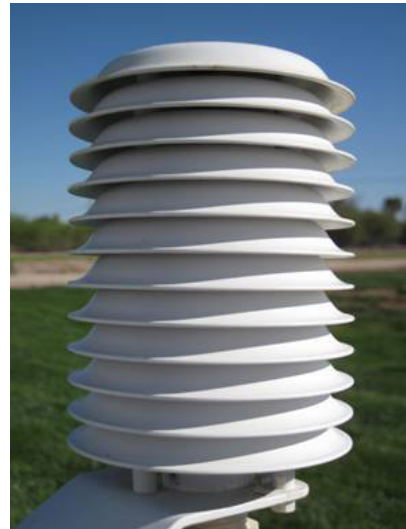
Figure 13. The Stevenson Screen (left) and the 12-plate Gill shield (right) are used to protect temperature sensors from radiation and precipitation. The temperature sensor should be installed at 5' (1.5m) above the surface.
