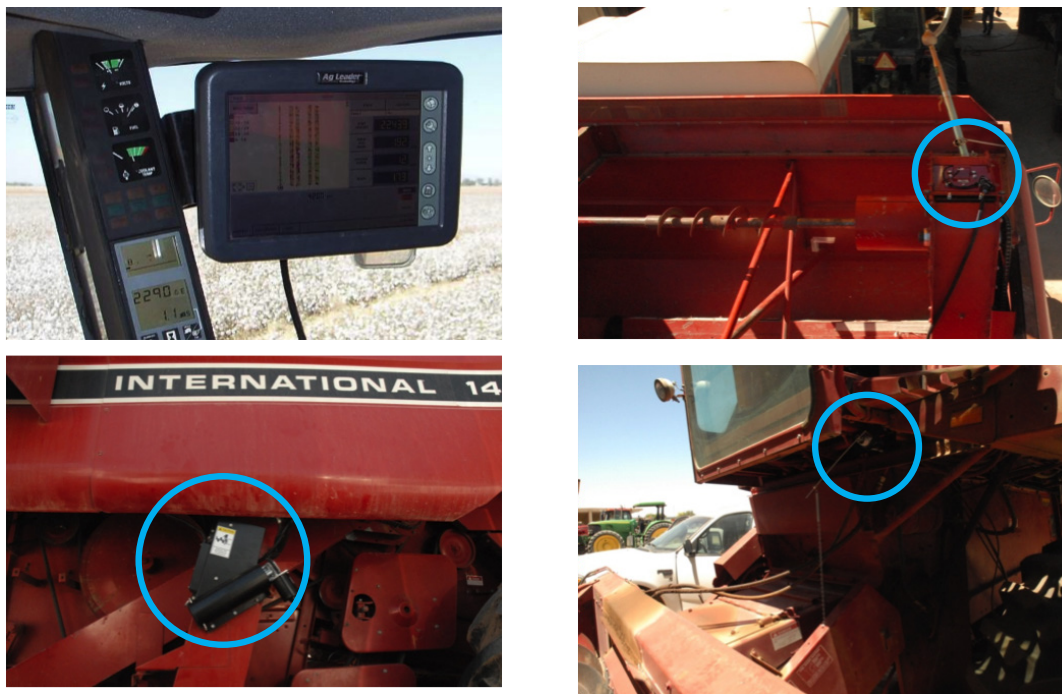
Figure 1. Yield monitoring system components in a yield monitor system installed on a conventional grain combine harvester (Case-IH 1440) in Central Arizona. From top-left corner in clockwise order: AgLeader Insight display; mass-flow sensor; header position sensor; and grain moisture sensor.
