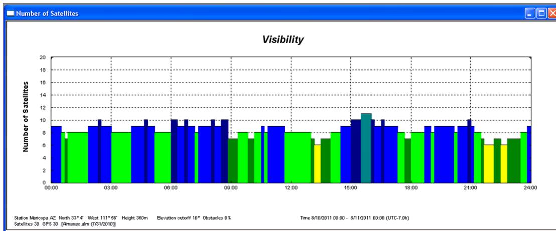
Figure 2. Predicted number of satellites visible in the Maricopa AZ area on August 10, 2011. Data generated with Trimble Planning Software v. 2.90.
