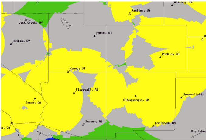
Figure 3. US Coastguard Radio Beacon stations providing differential correction service in Arizona. Yellow indicate areas covered by more than one station; gray areas are covered with one station; green areas have no coverage.
