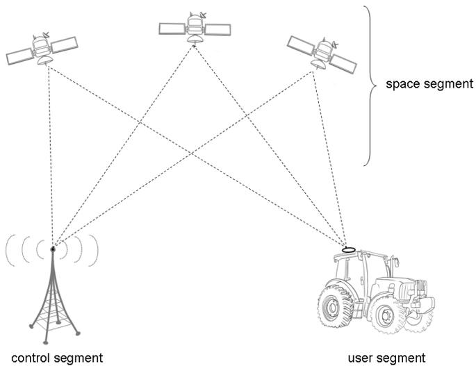
Figure 1. Diagram of GPS space, control, and user segments in agricultural applications.
