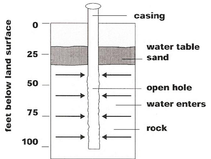
Figure 4. Casing depth in a bedrock and a sand-and-gravel well.
