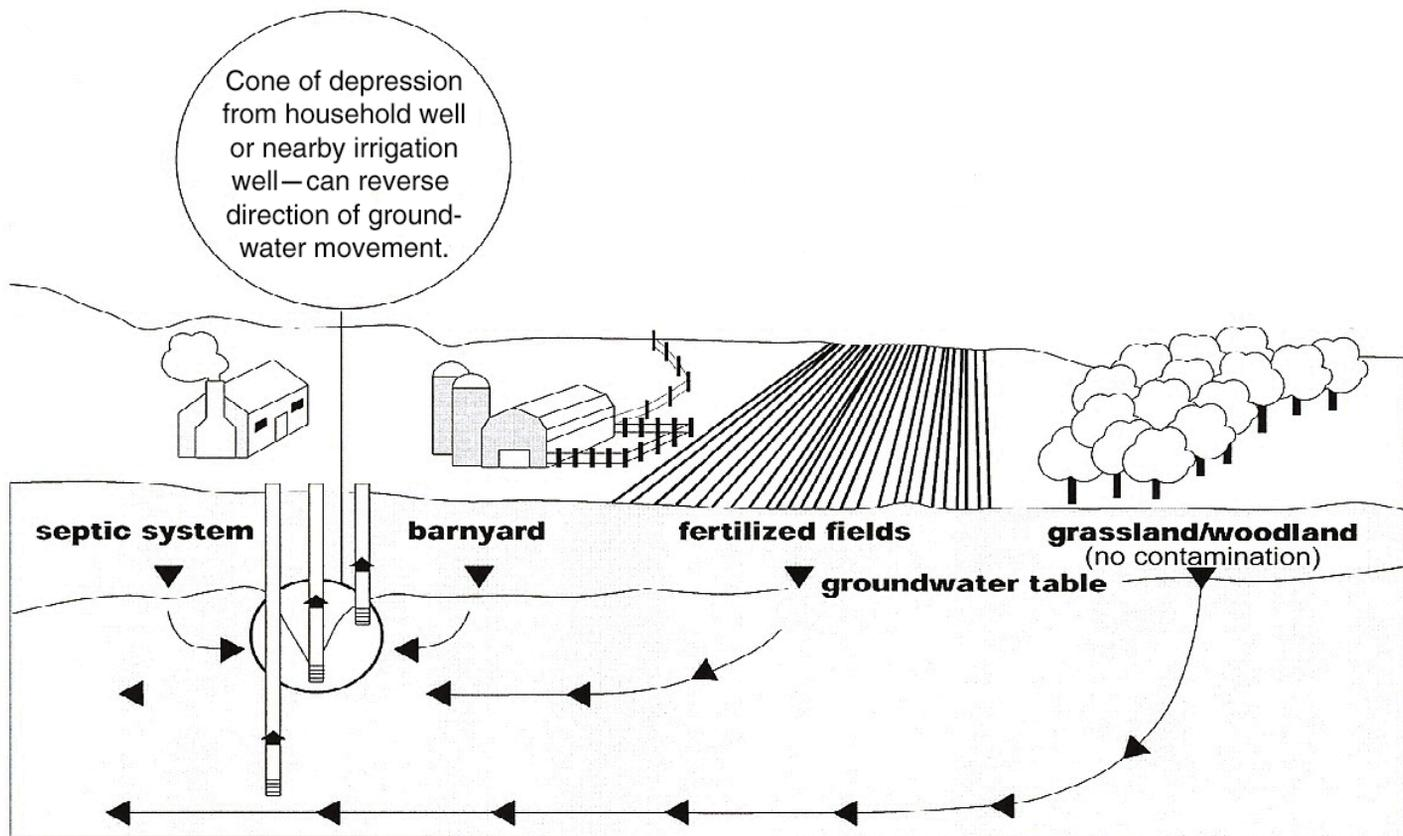
Figure 2. Direction of groundwater movement of a pumping system and potential sources of contamination.
