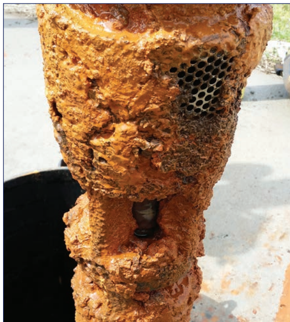
FIGURE 6.1 Buildup of biological slime and mineral crust on a submersible pump inlet. Photo provided by the National Groundwater Association.
