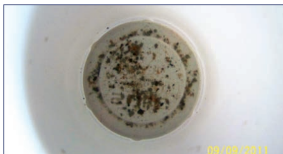
FIGURE 5.11 Sand and precipitated manganese particles, accumulated on the screen of an irrigation system.
