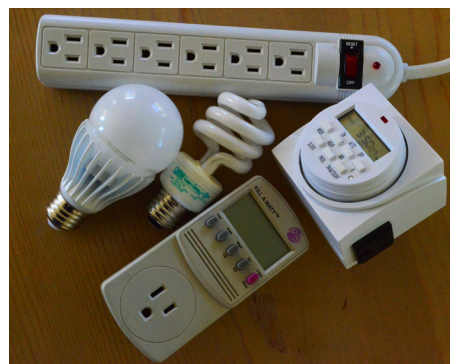
Figure 5. Home energy saving and monitoring devices: LED and CFL bulbs, power strip, timer, Watt meter.
