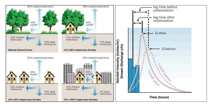
Figure 7. As impervious surface area increases in urban areas so does runoff (left graph). The increase in runoff leads to increased stream discharge (right graph). Base flow is not shown in this hydrograph (graph right) [from "Stream Corridor Restoration: Principles, Processes, and Practices, 10/98, by the Federal Interagency Stream Restoration Working Group (FISRWG)].
