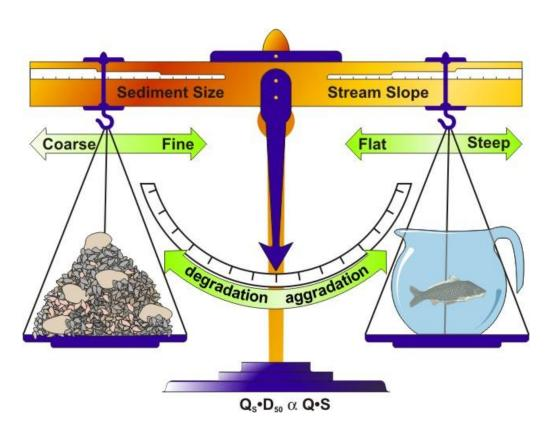
Figure 8. Relationship among stream discharge (Q), channel slope (S), sediment discharge (Q), and channel sediment size  $(D_{50}$  is the median grain size of the channel sediment) (Illustration by D. Cantrel modified from Rosgen, 1996).
