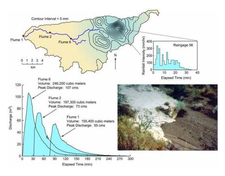
Figure 2. Summary of reduction in peak discharge associated with transmission losses as a flood flow travels through the Walnut Gulch channel (illustration by Carl Unkrich).
