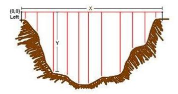
Figure 5. Schematic showing a general channel cross section, x indicates channel width and y indicates channel depth.
