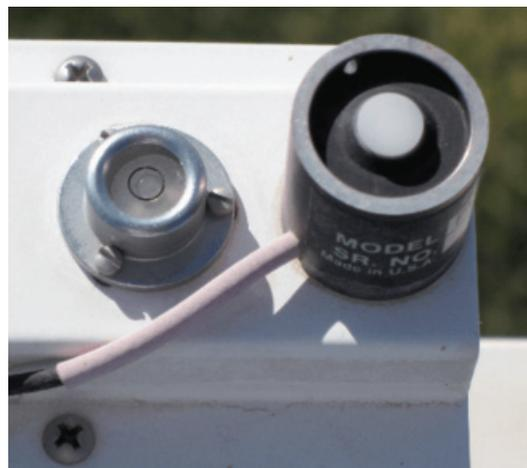
Figure 2. The silicon cell pyranometer is used to measure solar radiation on many automated weather stations.
