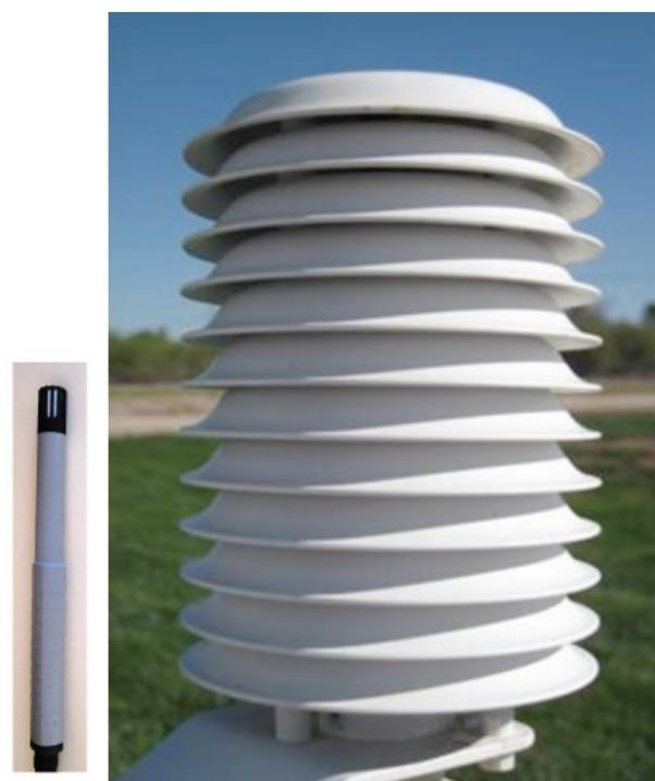
Figure 3. A combination temperature and relative humidity sensor (left) is housed within this radiation shield to protect the sensor from direct exposure to sunlight and rainfall.
