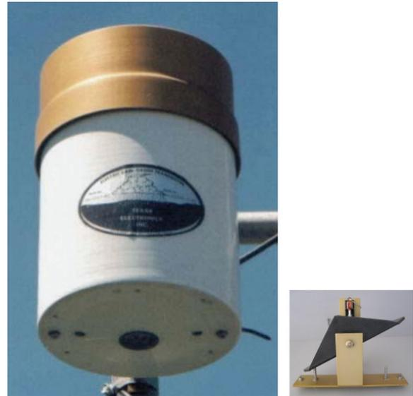
Figure 5. A tipping bucket rain gauge used to measure precipitation. The bucket mechanism (right) tips when a known volume of precipitation falls, triggering a switch closure which is recorded by the data logger.
