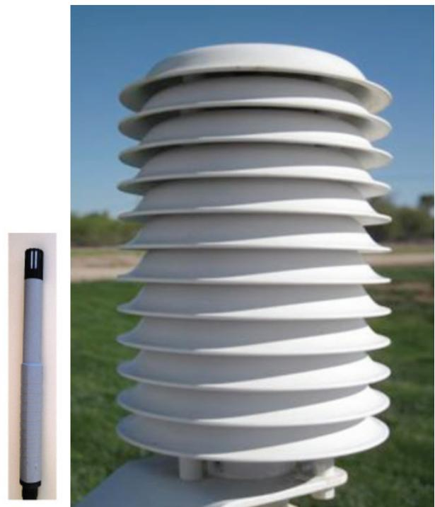
Figure 3. A combination temperature and relative humidity sensor (left) is housed within this radiation shield to protect the sensor from direct exposure to sunlight and rainfall.
