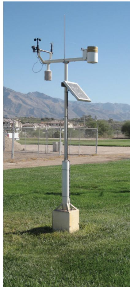
Figure 1. An automated weather station commonly used to estimate turf ET.
