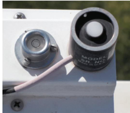
Figure 2. The silicon cell pyranometer is used to measure solar radiation on many automated weather stations.
