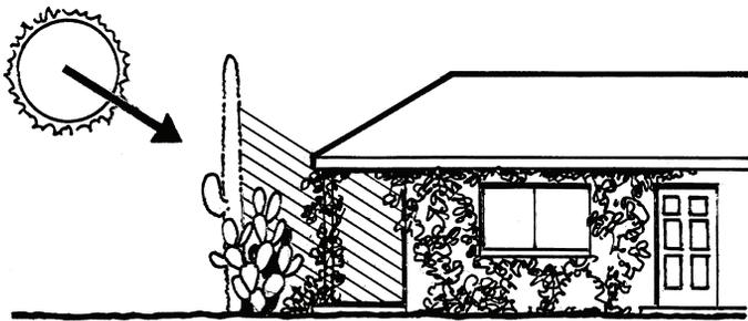
Figure 14: If tall trees are not possible, lower growing plants close to the building can provide temperature moderation.
