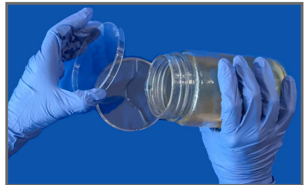
Pour until 3/4 of the bottom of the plate is covered, replace the lid and gently swirl the plate on the top of the table until the solution fully covers the bottom.
