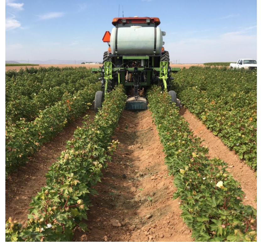
Weed-IT hooded sprayer in Arizona cotton. Field performance testing during 2020 season. UA-MAC.
