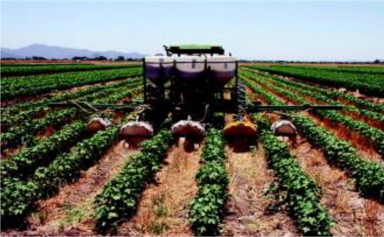
Weed-Seeker hooded sprayer in Arizona cotton planted after wheat. Conservation tillage in Arizona cotton. 2004 Agricultural Experiment Station Research Report.
