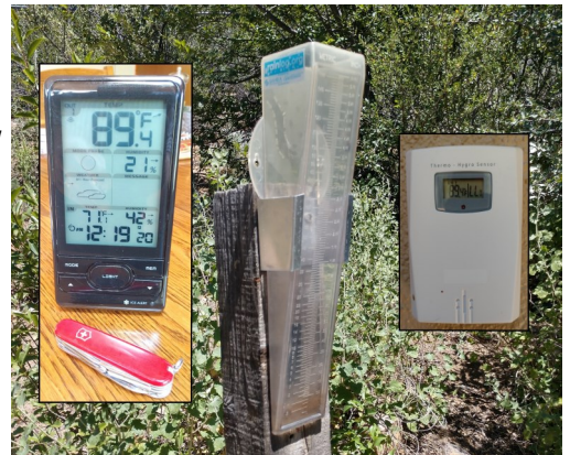
Wedge-type rain gauge (center) and max min thermometer (receiver in left and sensor on right) (Jeff Schalau, University of Arizona).
