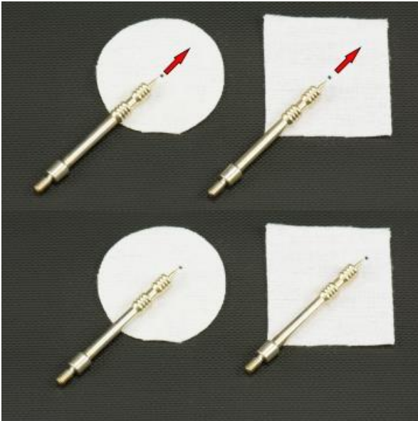
Figure 2: Proper Side Spiking Location
