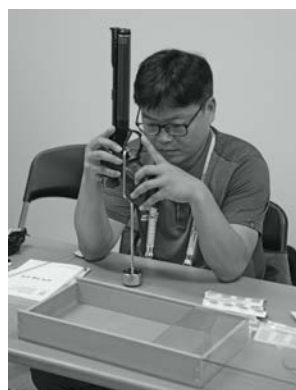
Proper trigger weighing technique is shown in this photo. Both elbows must be on the table as the pistol is lifted with the 500 g weight.
