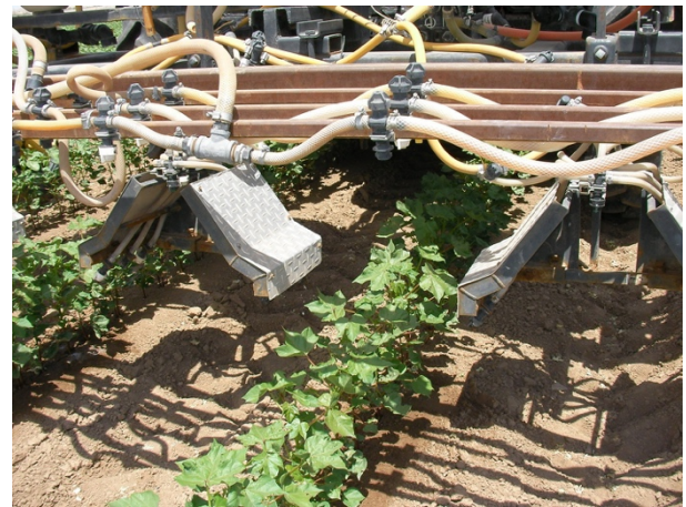
Figure 4. Post-emergence stem drench application technique.
