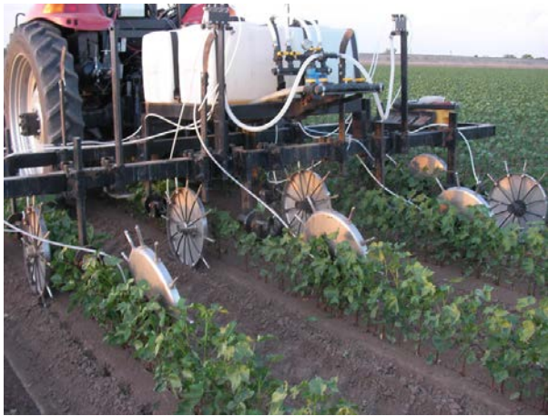
Figure 3. Post-emergence point injection application technique.
