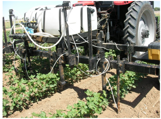
Figure 2. Side dress application technique utilizing an injection knife.
