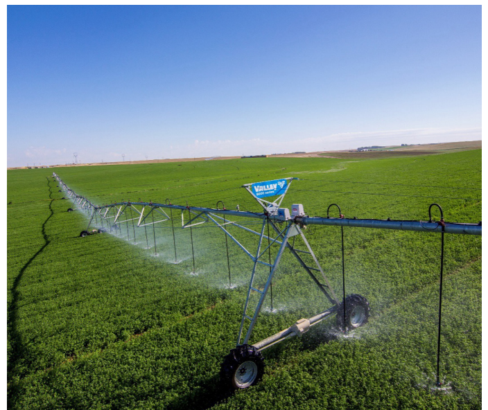
Figure 10. Center pivot nozzles in action. Image credit: Valmont Industries ( https://www.valleyirrigation.com/ ).
