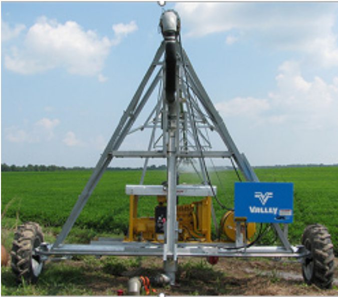
Figure 7. Center pivot tower requires regular checking and prompt maintenance. Image credit: Valmont Industries (Valmont Industries, 2015, https://www.valleyirrigation.com/ ).
