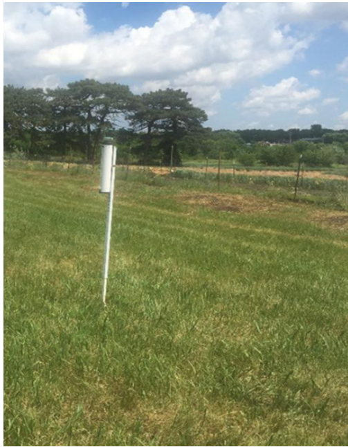
Figure 5: ETgauge® atmometer placed in the field to estimate reference evapotranspiration by measuring evaporation from a porous ceramic surface.
