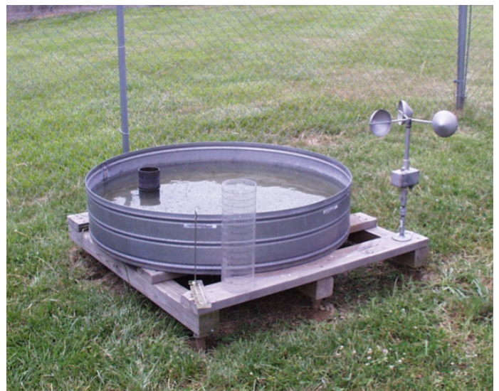
Figure 4: Standardized evaporation pan placed in the field to measure atmospheric evaporative demand.
