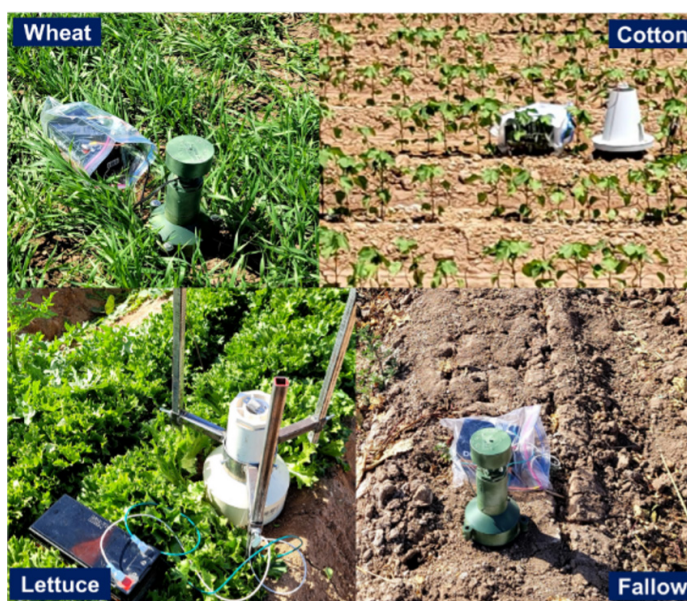
Figure 2. In-situ soil CO 2 sensor deployment in different commercial crop fields and fallow grounds for comparisons
