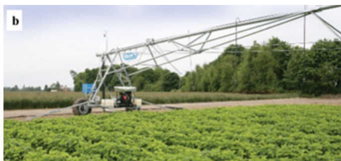
Figure 2. (a) Center pivots and (b) linear move systems. (Credit: Valley [Valmont] Company. Used by permission)
