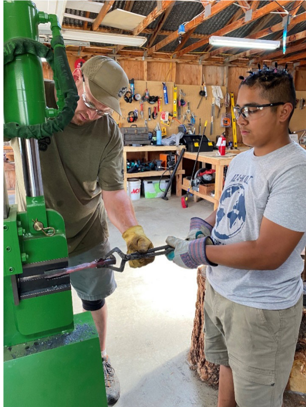
Figure 2: Using a forging press. Eye protection and gloves are used, in addition to tongs to keep hands away from the heat and press jaws.
