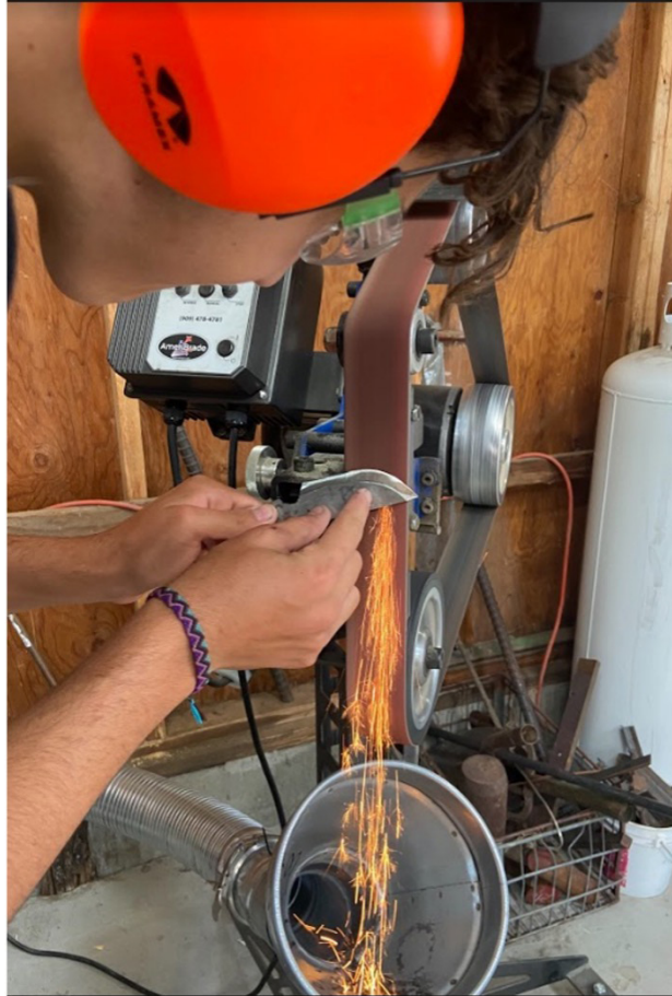
Figure 5: Grinding a knife from high carbon steel. Note the “firework” sparks - these bright exploding sparks are a good indicator of high carbon amounts in steel.
