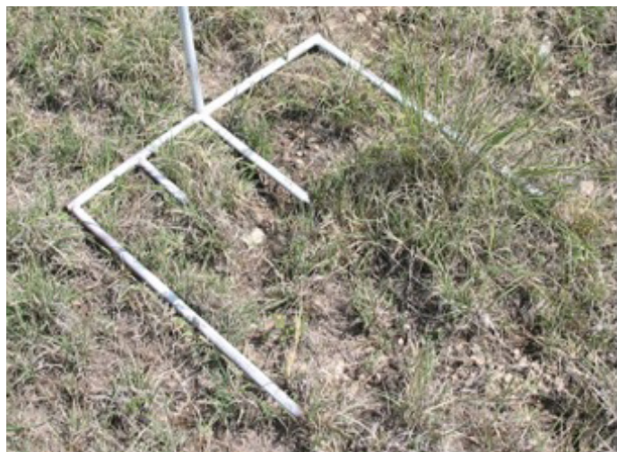
Photo 2. A "nested" sampling frame which can be used as a 10-, 20-, or 40-cm 2 quadrat. Photo credit, George Ruyle.
