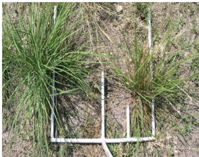
Photo 2. A "nested" sampling frame which can be used as a 10-, 20-, or 40-cm 2 quadrat. Photo credit, George Ruyle.
