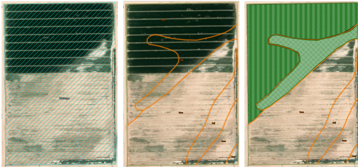
Figure 2. USDA-NRCS Web Soil Survey maps with imagery as background of a 56-acre field in SW Arizona. Image on the left depicts the field and associated area of interest (AOI); diagonal lines indicate the geographic extent of the field. Image on the center shows contour lines and areas of soil units present in this AOI. The image on the right shows an arbitrary example of creating two management zones in the area with more fertile soil units.
