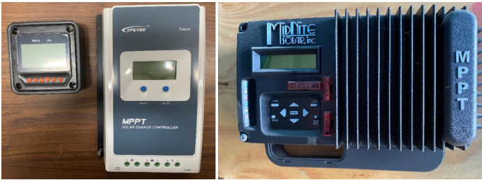
Figure 10. Examples of multi power point tracking (MPPT) charge controllers. Source: Author
