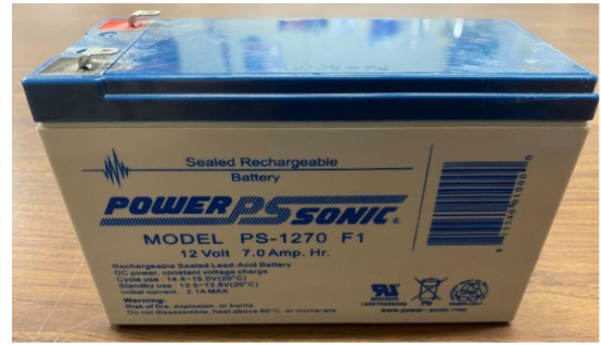
Figure 12. Example of a sealed lead-acid solar battery. Source: Author
