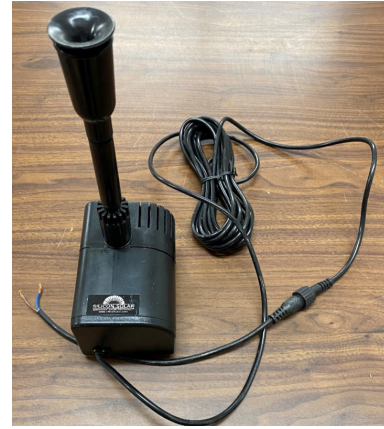
Figure 19. Example of a direct current load: 12V solar-powered water fountain. Source: Author.
