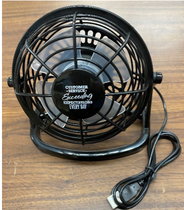
Figure 16. Example direct current load: 12V fan. Source: Author.
