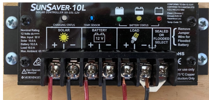
Figure 7. A 10-amp, 12-volt, PWM-type charge controller. Source: Author.
