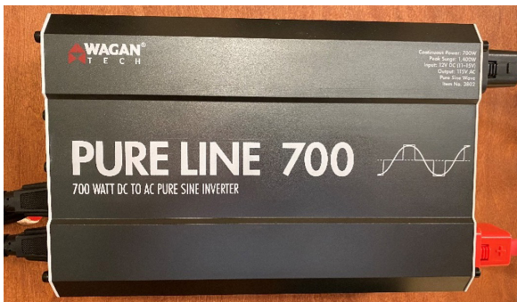
Figure 22. Example of a pure sine wave battery inverter with a 700-watt capacity. Source: Author.
