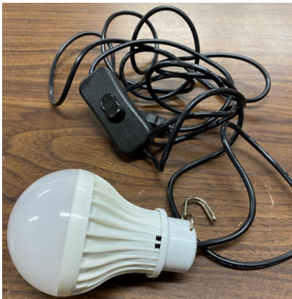
Fig 18. Example a direct current load: 12V light with USB connection. Source: Author.
