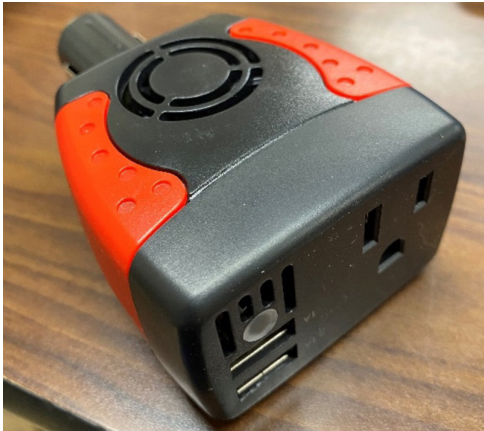
Figure 21. Example of a smaller-sized DC inverter plugs into a 12V power socket. Source: Author.
