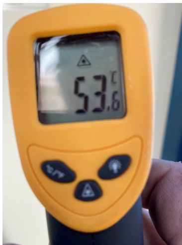
Figure 22. A non-contact thermometer is used to measure the surface temperature on a solar module. Source: Author
