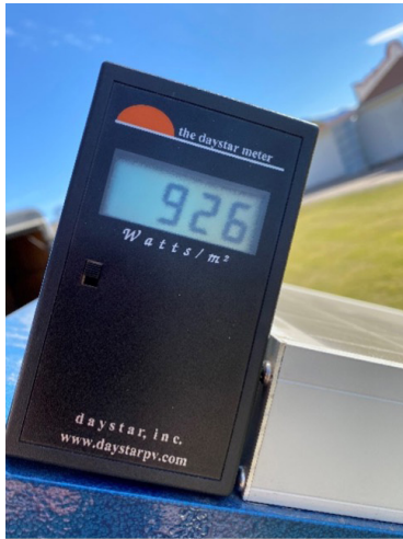
Figure 21. Pyranometer measures sunlight intensity in Watts/m 2 . Source: Author.
