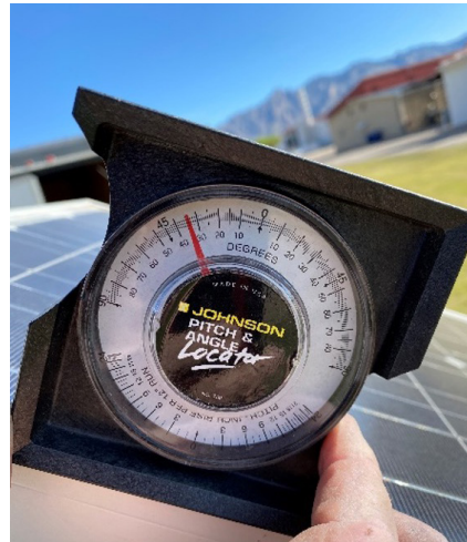
Figure 20. Angle finder reveals the tilt-angle of the solar module. Source: Author
