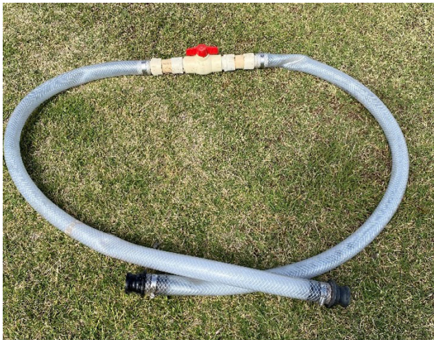
Figure 13. Reinforced poly tubing return line. Source: Author
