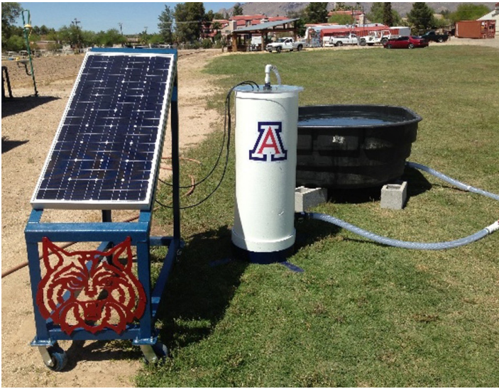
Figure 1. Mobile Solar-Powered Water Pumping Demonstration System. Source: Author
