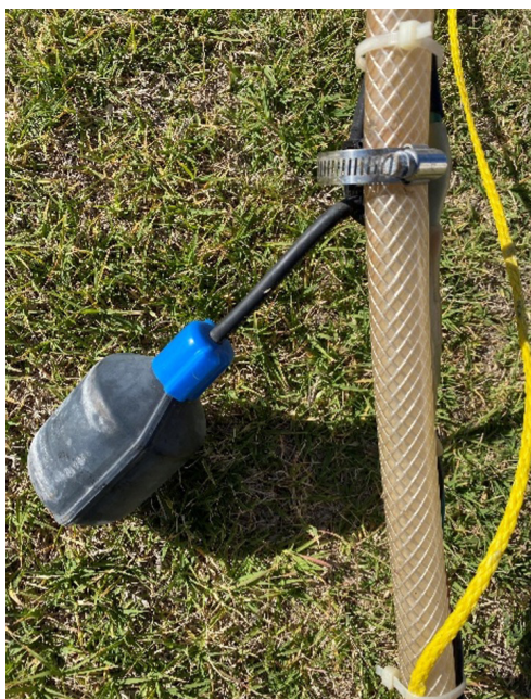
Figure 9. Float switch used in a low water cut off application in the well. Source: Author
