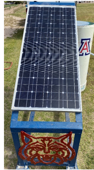
Figure 2. A solar module mounted in a fixed position on a mobile frame. Source: Author
