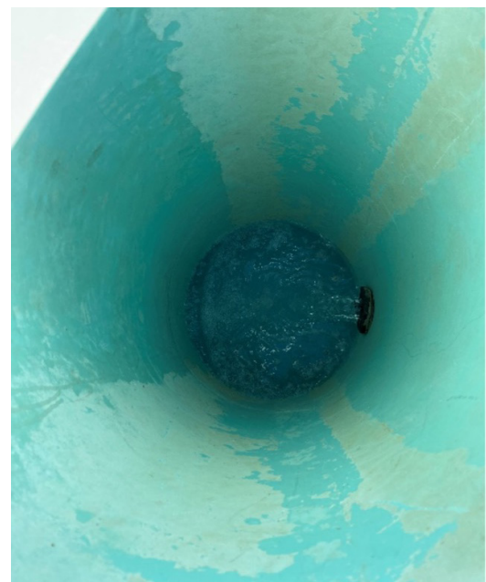
Figure 10. Float switch used in a low water cut off application in the mock well cistern Source: Author
