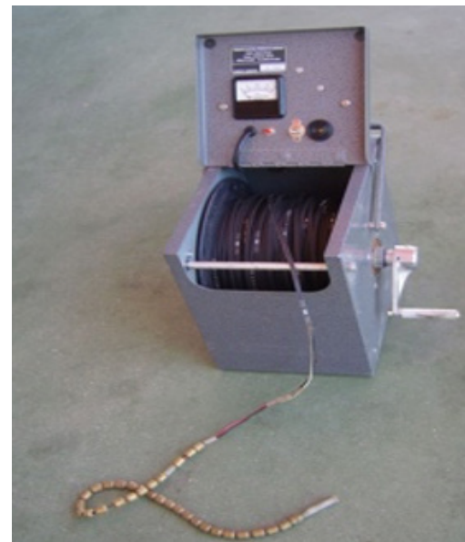
Figure 1. A Powers Electric 500-foot sounder. No endorsement implied. Source: G. Hix
