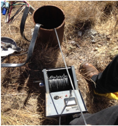
Figure 5. Sounding a pitless adapter well with cover cap removed. Source: G. Hix
