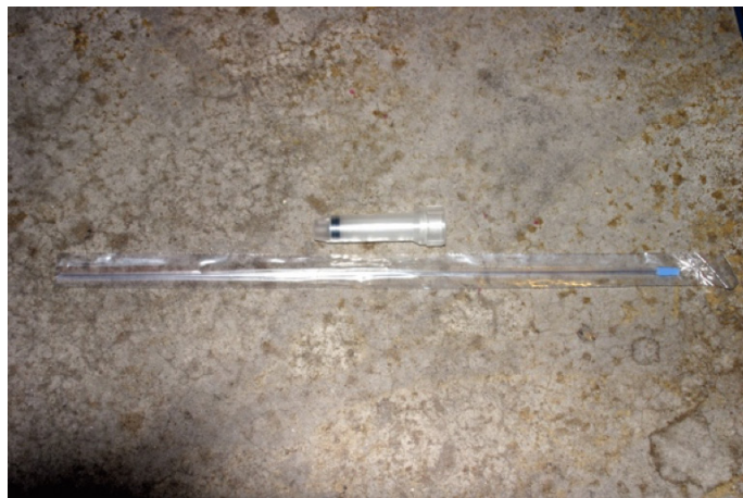
Figure 2. Pipette and Syringe set up for sampling
