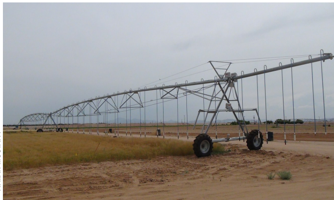
Figure 4. Lateral move pivots irrigate a crop in Maricopa, AZ. By applying water with overhead sprinklers, the irrigation water and other inputs such as fertilizers can be delivered more precisely than with flood irrigation.
