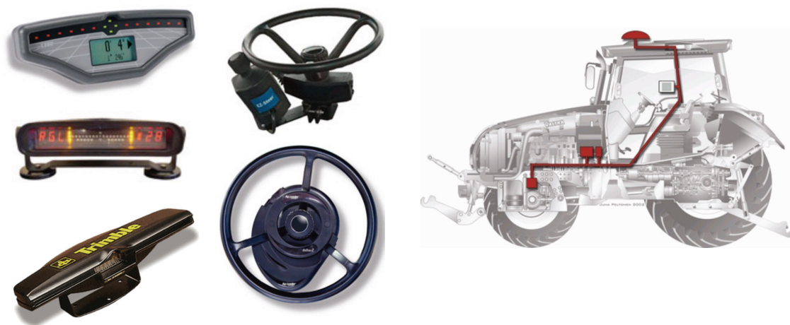
Figure 3. Examples of GPS-based steering control. Left column shows three examples of dash-mounted light-bar systems, center column has two cases of steering assist, and drawing on the right depicts an auto-pilot system with fully-integrated steering control.
