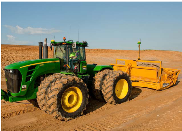
Figure 6. GPS-based land leveling solutions. On the left is John Deere i-Grade, and the right picture displays Trimble AgGPS FieldLevel II.
