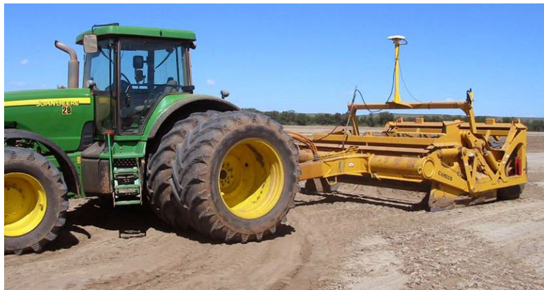
Figure 6. GPS-based land leveling solutions. On the left is John Deere i-Grade, and the right picture displays Trimble AgGPS FieldLevel II.
