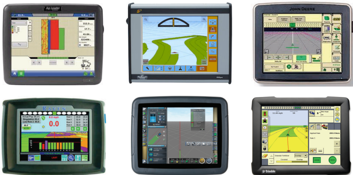
Figure 2. Examples of multifunction displays currently available for tractors, sprayers and other agricultural machines. In clock-wise order beginning from the top-left: Ag Leader Integra, Hemisphere Outback S3, John Deere GS3 2630, Raven Envizio Pro II, Topcon X30, and Trimble AgGPS FmX.
