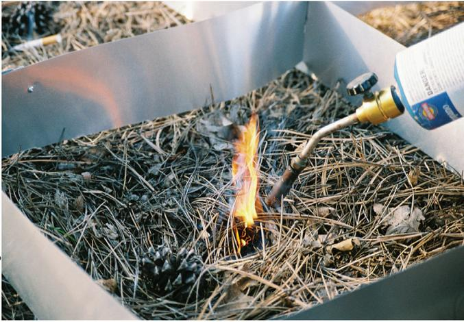
Figure 2. Propane torch igniting the pine needles.
