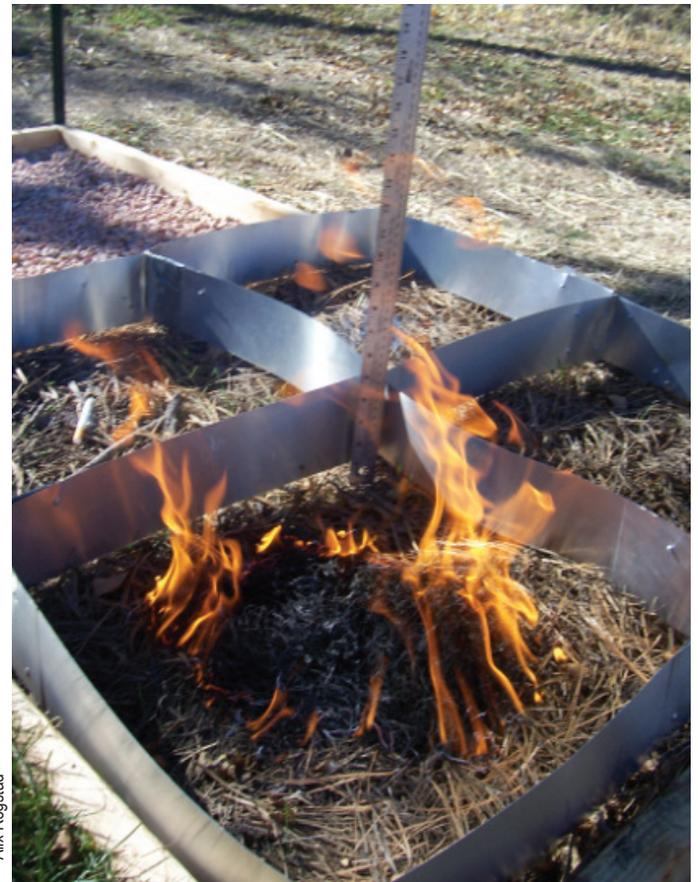
Figure 3. Measuring flame length in the ¼ meter cell with a metal ruler.
