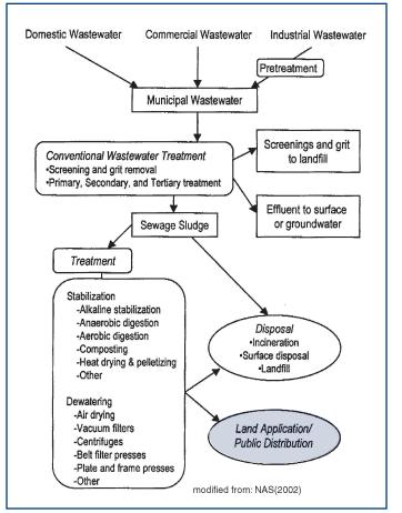
Figure 1. Municipal Wastewater and Sewage Sludge (Biosolids) Treatment Options. Source NAS(2002)
