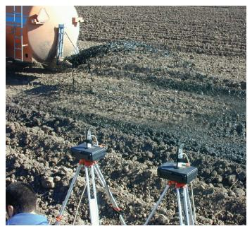
Figure 3. Land application of liquid biosolids via a spray applicator. Source: Environmental Pollution Science (2006) chap.23.
