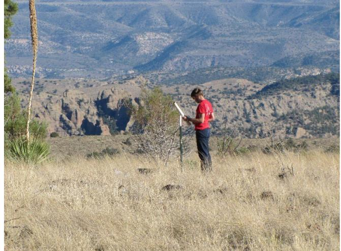
*Reading and recharging a remote rain gauge on 4 Bar Mesa.*
