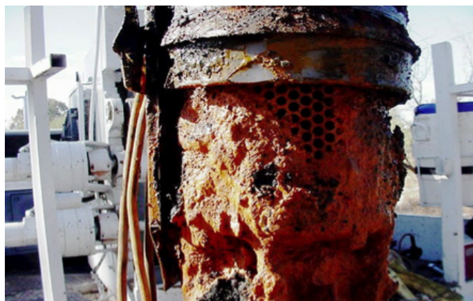
Figure 6. A well pump intake screen covered with red slime and iron rust formed by bacteria living inside a pumping well. Photo by G. Hix.
